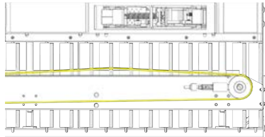
Figure 83: Proper Belt Tension
