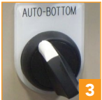
3 Top & bottom or bottom only seal operation modes
