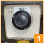
1 "Clear" button for jams & replacing bottom tape roll (Opposite Side of Machine)
