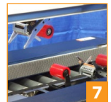
7 Offset tape heads process 2" high cases
