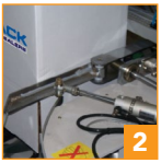
2 Pneumatic arm squares cases before sealing
