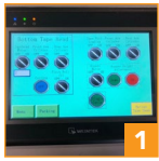
1 Automatic and Manual mode operation with failure diagnostic LED readout
